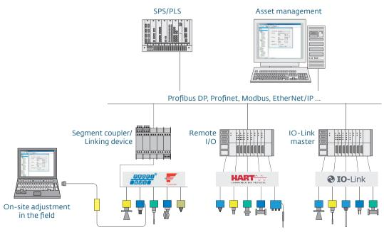
Communication-capable field instruments
