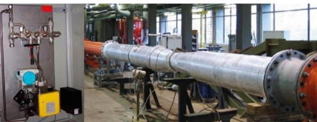
measurement with venturi measuring section, for billing of steam
